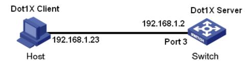
Figure 108: Dot1x configuration example
