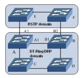
Figure 59: RSTP Transparent Transmission Application
