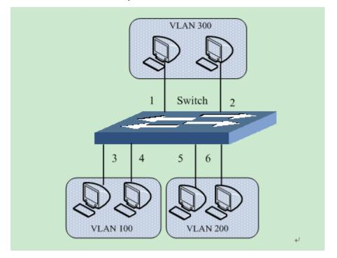
Figure 129: PVLAN Configuration Example
