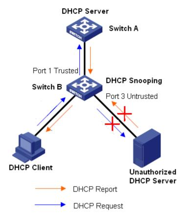
Figure 174: DHCP Snooping Typical Configuration Example
