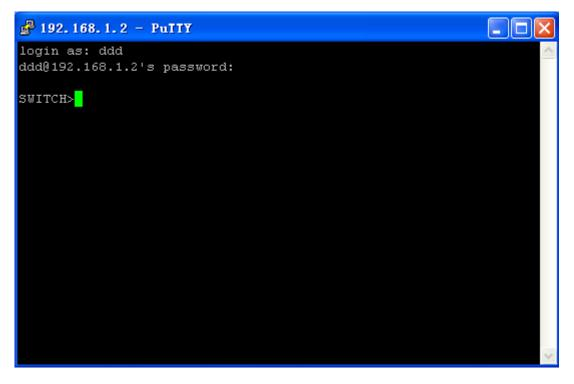
Figure 97: Login interface of the SSH password authentication
