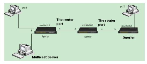
Figure 79: IGMP Snooping Application Example
