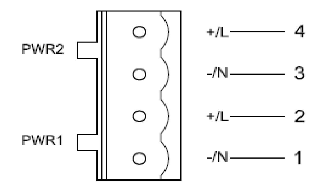
Figure 12 4-Pin 5.08mm-Spacing Plug-in Terminal Block (socket)
