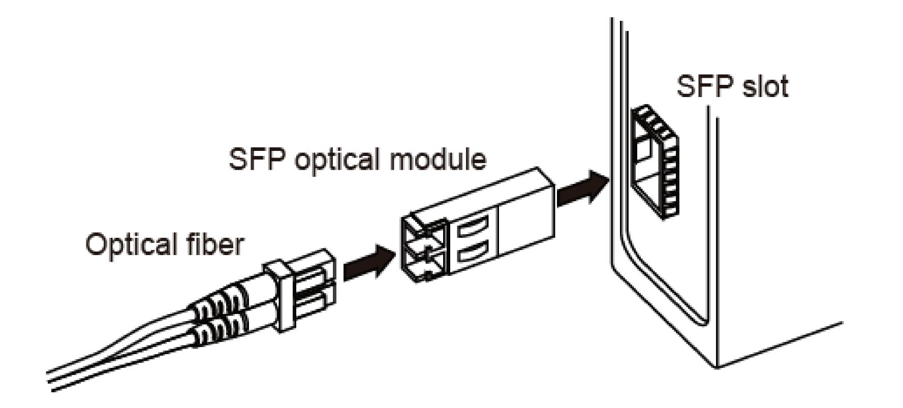
Figure 11 Connecting the SFP Optical Module
