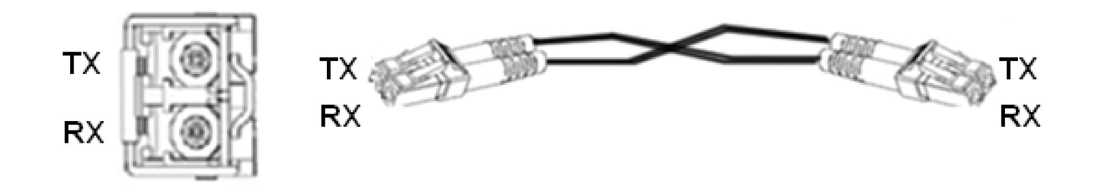
Figure 10 Fiber Connection of an SFP Optical Module
