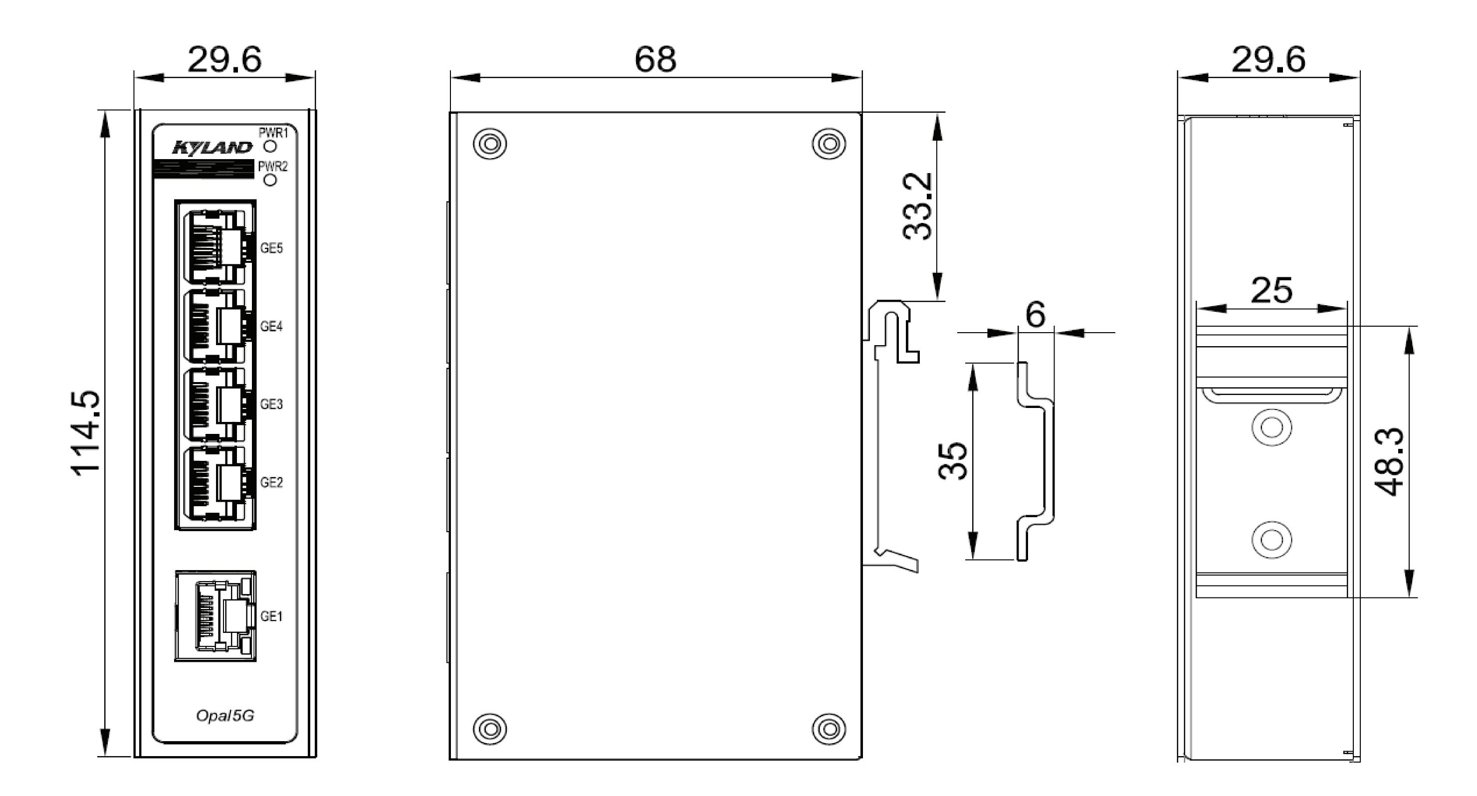
Figure 3 Opal5G Dimensions for DIN-Rail Mounting (unit: mm)
