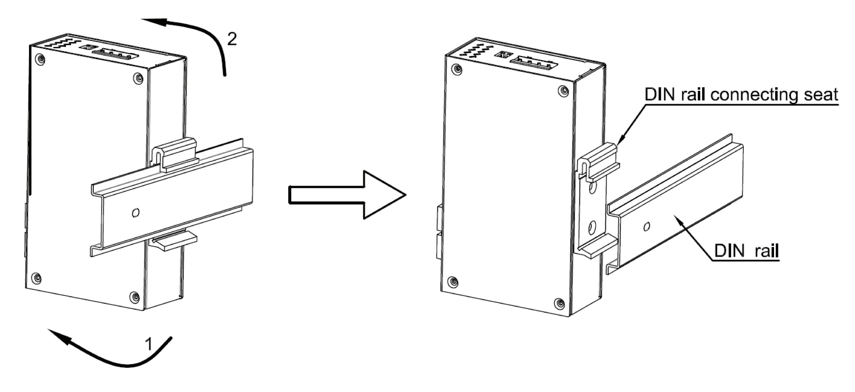
Figure 6 DIN Rail Dismounting
