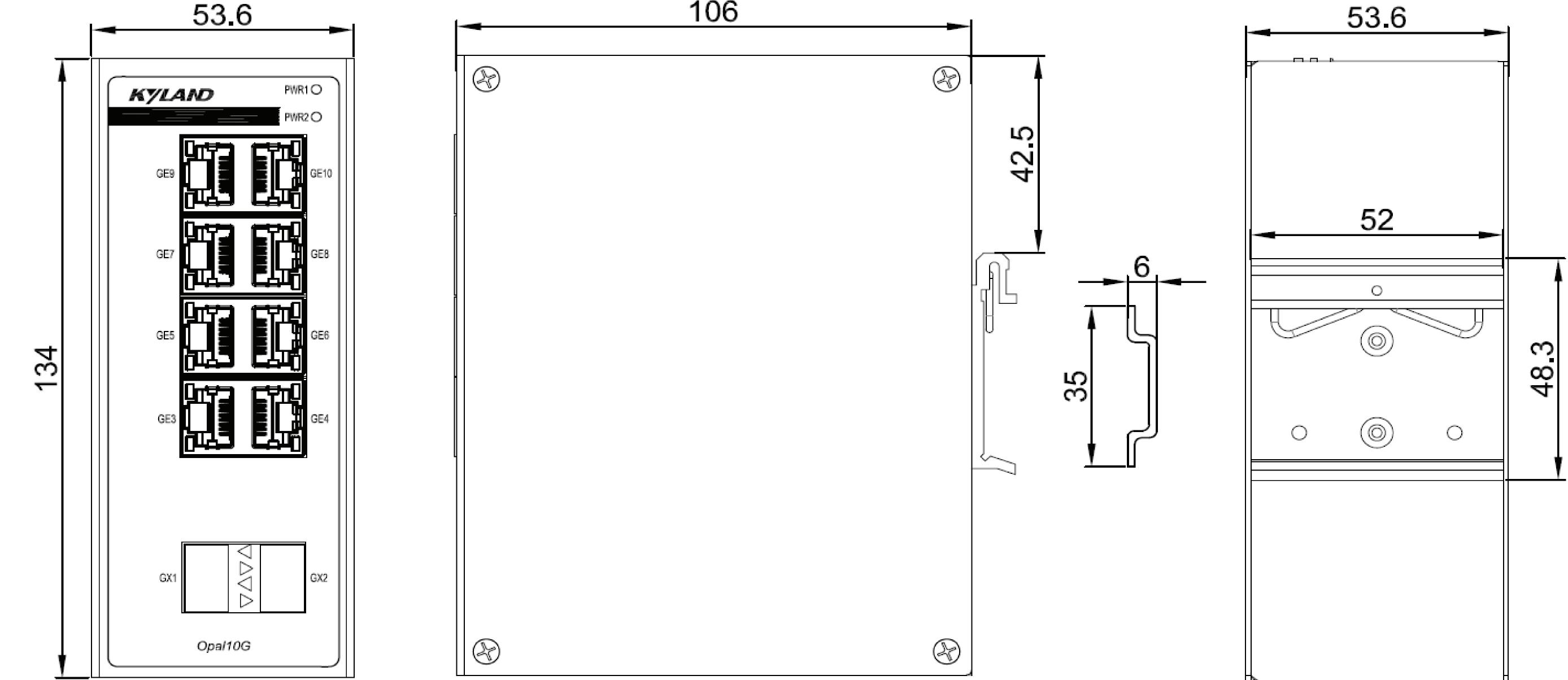
Figure 4 Opal10G Dimensions for DIN-Rail Mounting (unit: mm)
