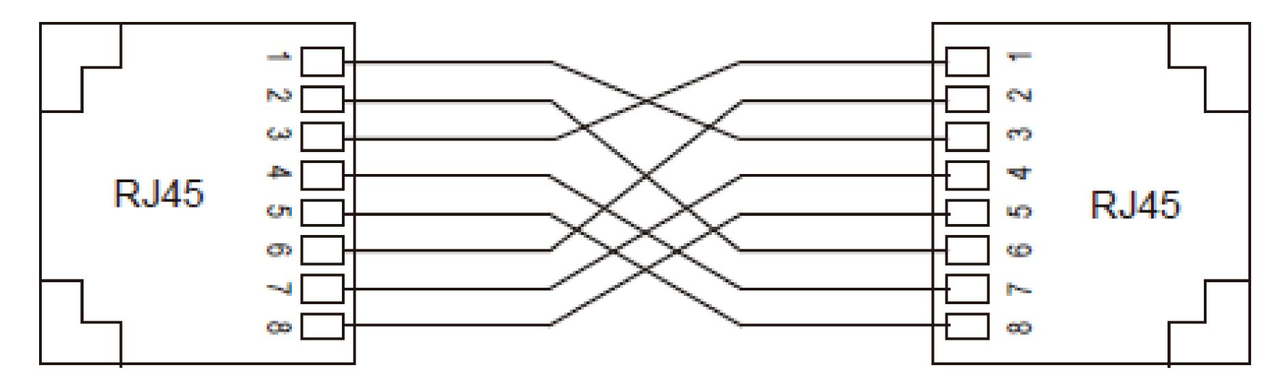
Figure 8 Connection Using Straight-through/Cross-over Cable
