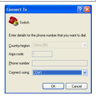
Figure 3 Selecting the Communication Port
