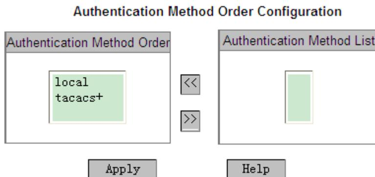
Figure 120: Configure authentication method
