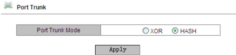
Figure 43: Port Trunk Mode Setting
