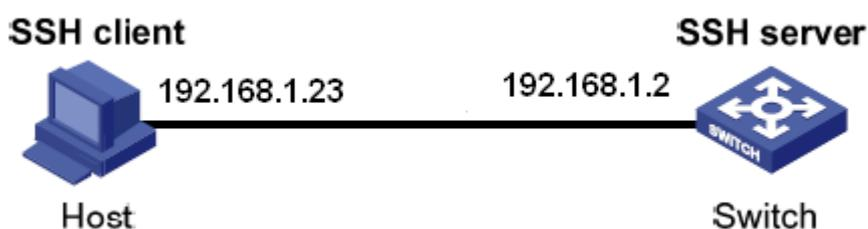
Figure 102: SSH configuration example
