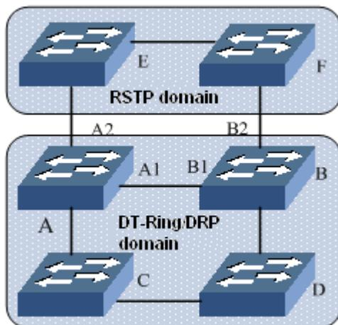
Figure 63: RSTP Transparent Transmission Application
