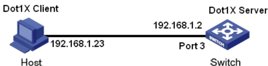
Figure 116: Dot1x configuration example
