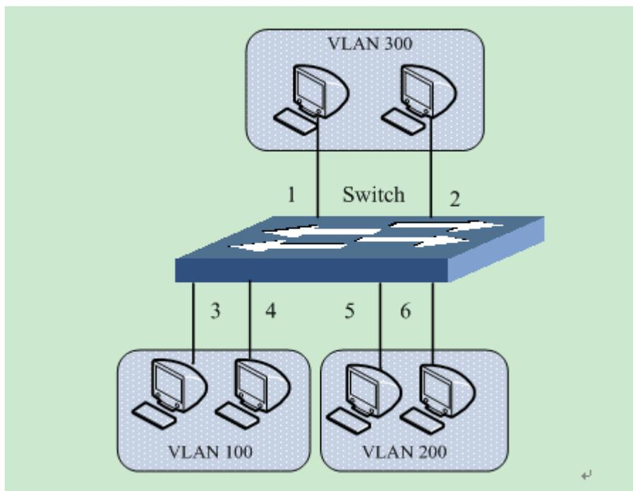
Figure 137: PVLAN Configuration Example
