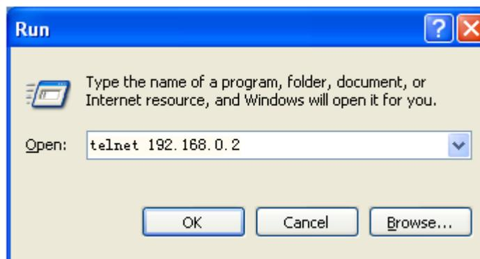
Figure 6: Telnet Access
