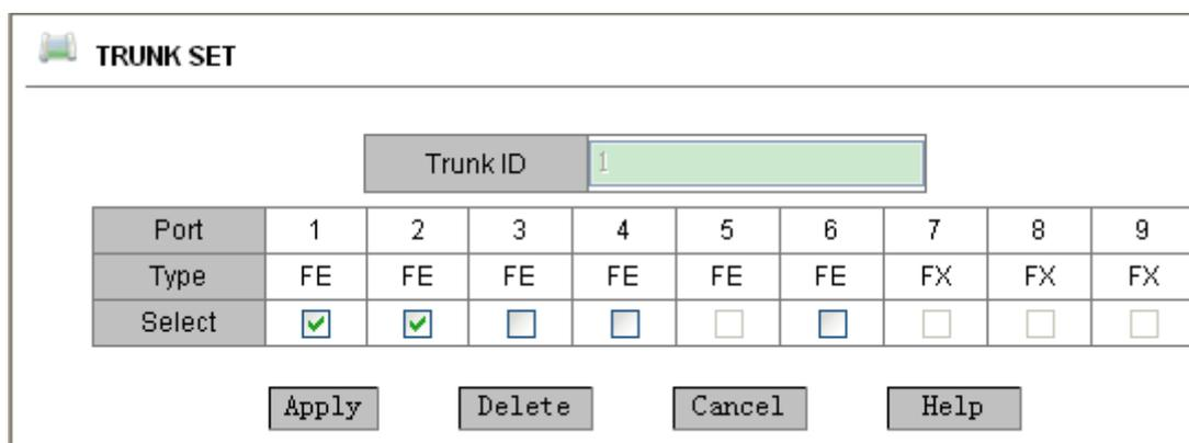
Figure 46: Detailed configuration of Trunk Group
