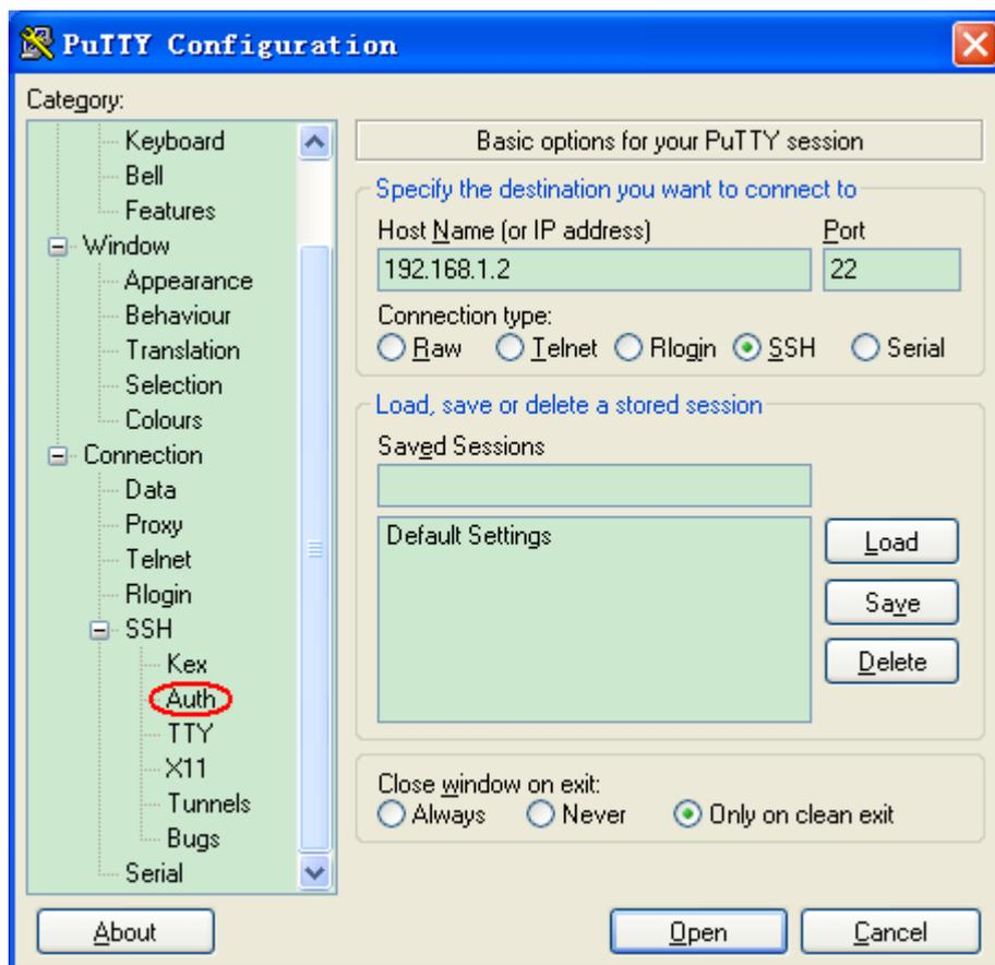
Figure 109: SSH client configuration of the "Public Key" authentication
