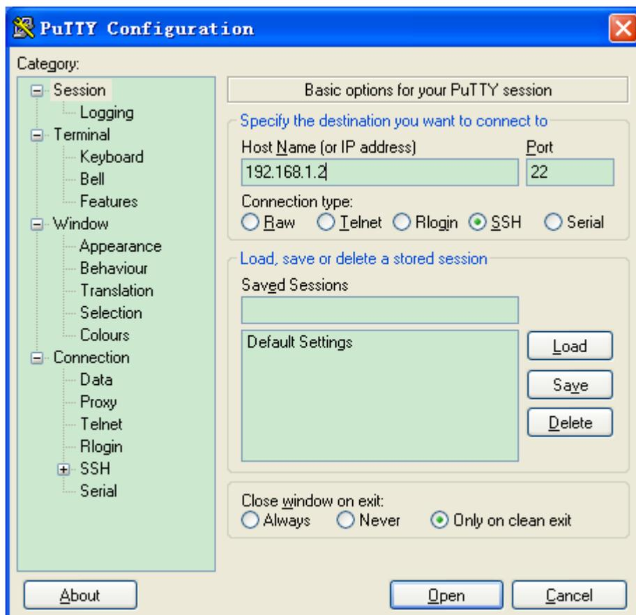
Figure 103: SSH client configuration
